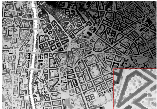
Fig. 3: DSM computed from 155 images of the Graz dataset; Note the enlargement at the lower right.
