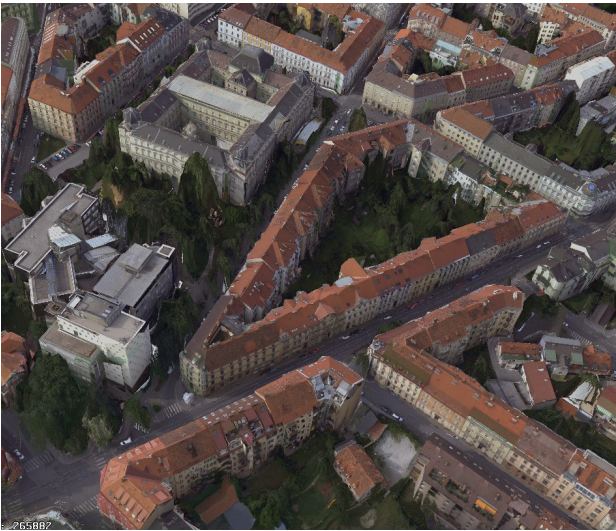
Fig. 12: Reconstructed buildings placed into textured DSM; visualised region is marked red in Fig. 7
