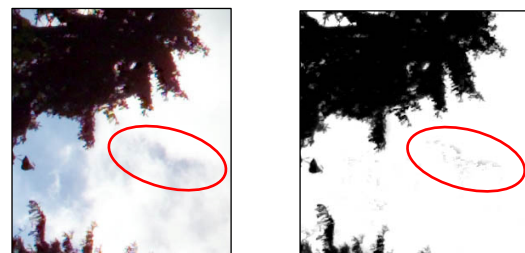
Figure 13. Original image with clouds (left) and classified image with fragments caused by cloud borders (right)
