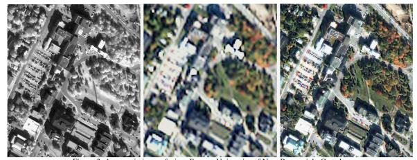
Figure 3. Automatic image fusion, Ikonos, University of New Brunswick, Canada. Left: Original panchromatic image (1 m); Center: Original natural colour image (4 m); Right: Fused natural colour image (1 m).
