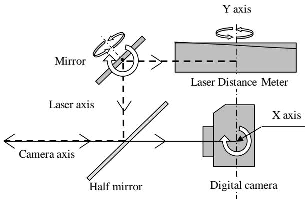
Figure 2. Configuration of the system
