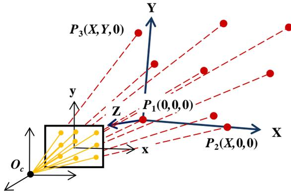
Figure 5. Coordinates system of the IBIM system
