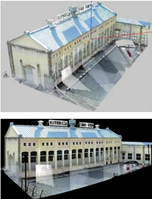
Figure 4. Top: Scanned Data (3D) Bottom: Range Image (2D)
