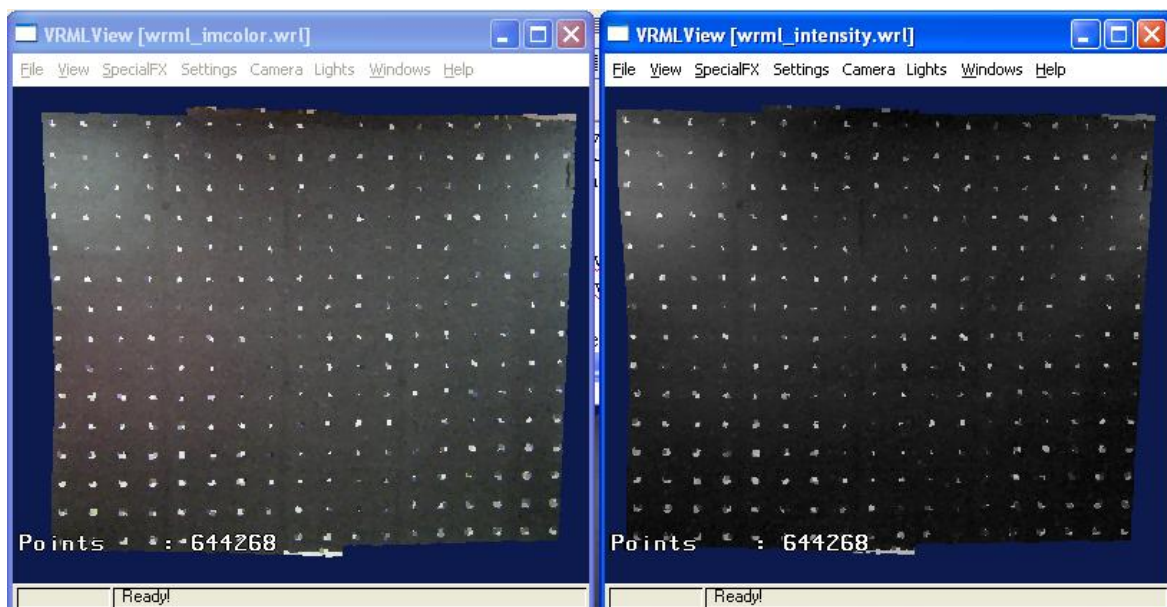
Figure 4. Laser scanning points with image colours and TLS intensities.
