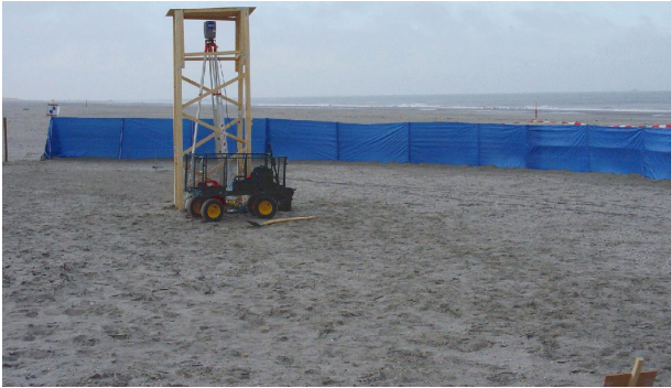
Figure 1: Experiment setup: sand particles transported towards the plastic screen and the wooden house protecting the terrestrial laser scanner Faro Photon 120.
