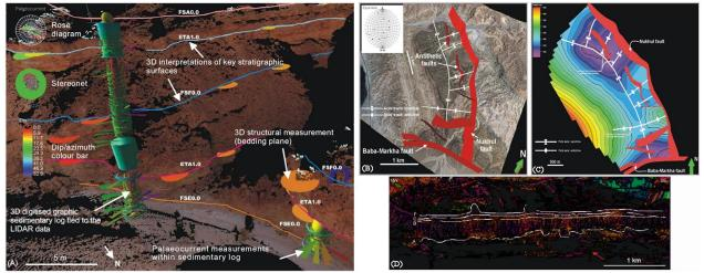
Figure 1. (A) Point cloud coloured by digital photos, providing a georeferenced framework for integrating field observations. (B-D) Fault models developed from 3D outcrop model. The stereonet shows poles to fault planes derived and (C) a structure contour map of key stratigraphic horizon generated for the Nukhul half-graben.
