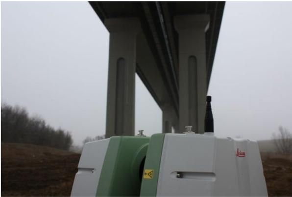
Figure 6: Scanning station underneath the Szebényi Bridge
