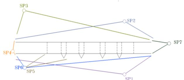
Figure 2. Different scan positions and field of view from each station around the bridge.
