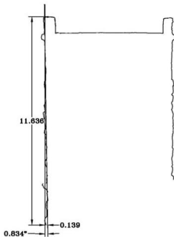
Figure 6. Deformation in the right downstream wall in a transversal section of the bridge.
