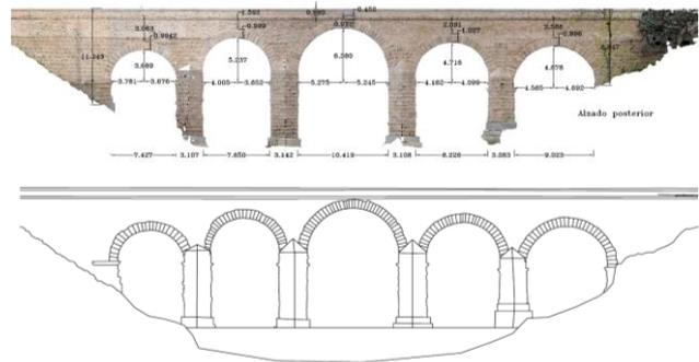
Figure 4. Orthophoto and plane of the upstream wall.
