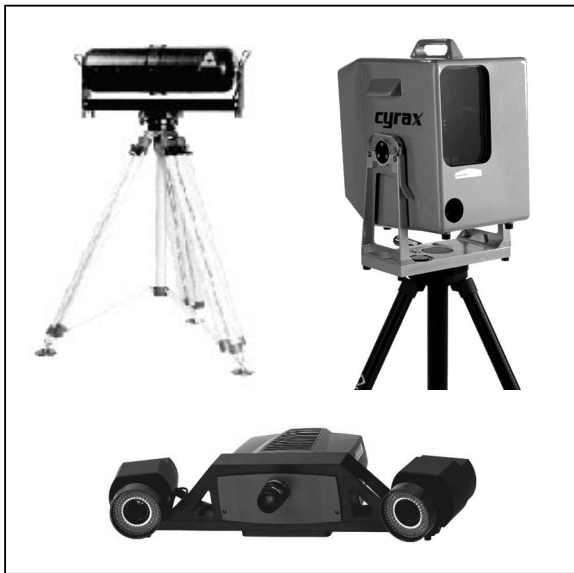
Figure 1. Scanners: Mensi S25 (top left), Cyrax 2500 (top right), GOM ATOS II (below)
