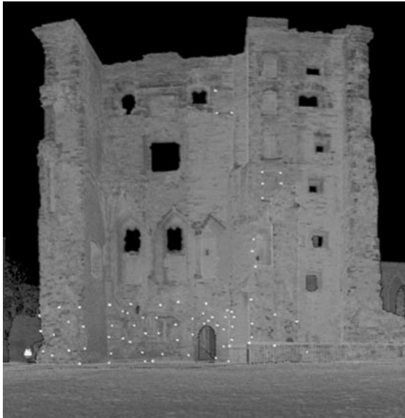
Figure 2. A sub-section of the intensity image produced by the Riegl LMS Z210 scanner.
