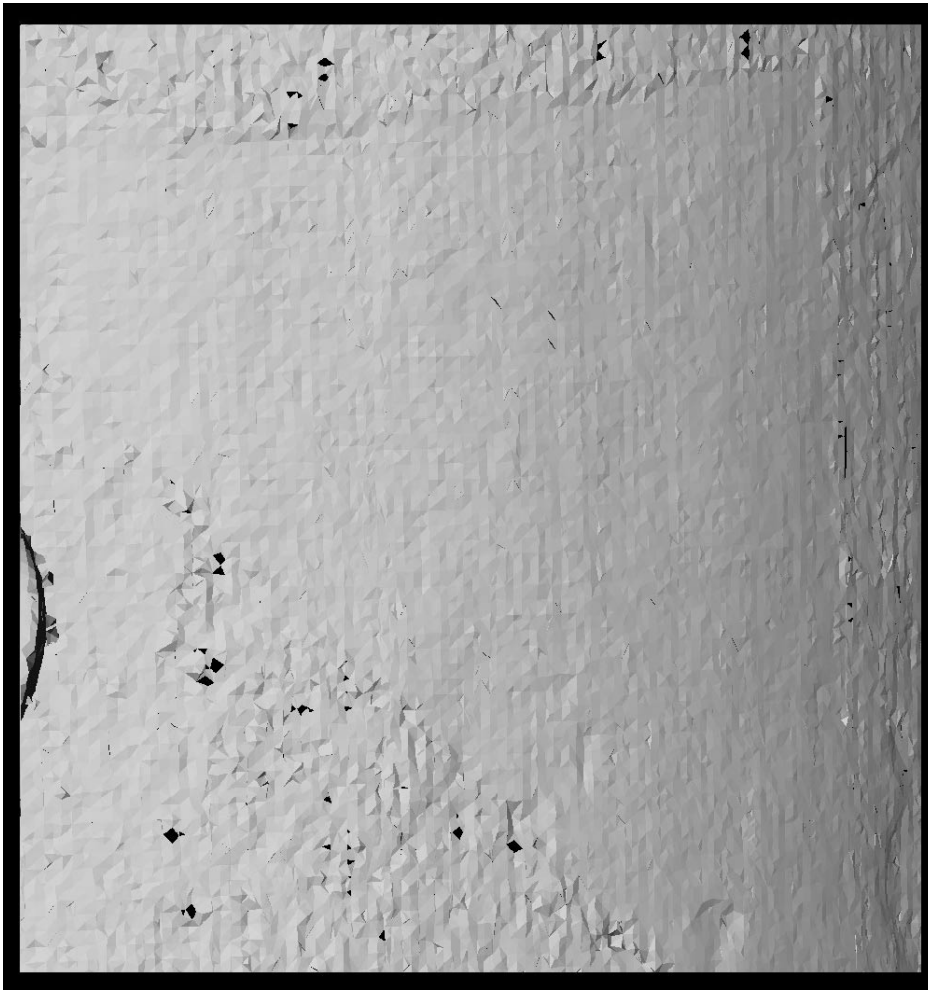
Fig. 8 Detail (Fig.7): denser cloud of points produces smoother surface when meshed
