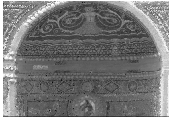
Fig. 13 - House of the Small Fountain: particular of orthophoto obtained by using surface model provided by laser scanning.
