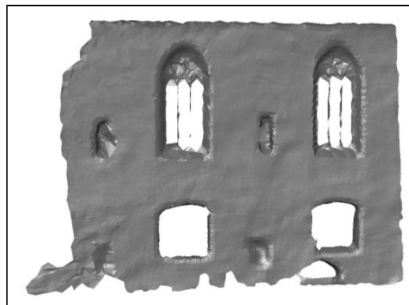
Figure 3. Polygonal model as a basis for an orthophoto
