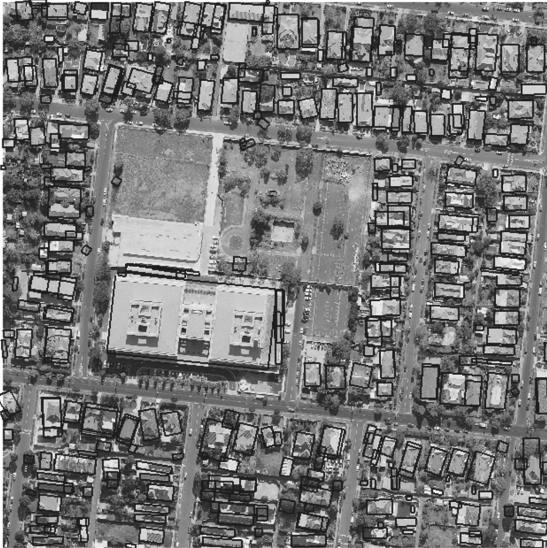
Figure 13. Building detection by the improved algorithm on a scene from Moonee Ponds.
