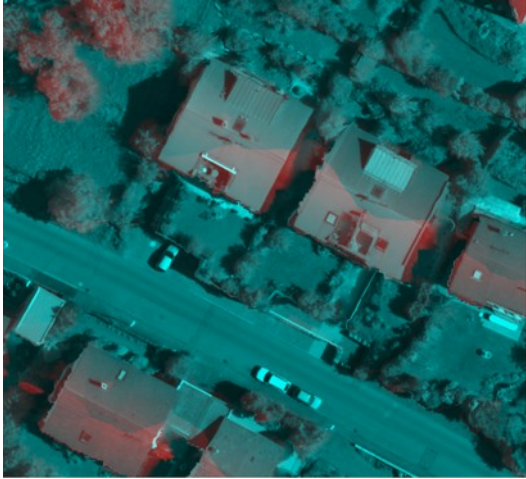
Combined image: Red channel is normalised height, green and blue: intensity from CIR
