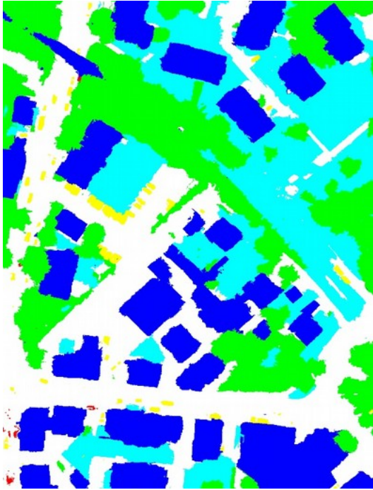
Figure 8: Results from SVL_3: SVL-features, including NDVI, saturation and normalized height, but only boosting classification
