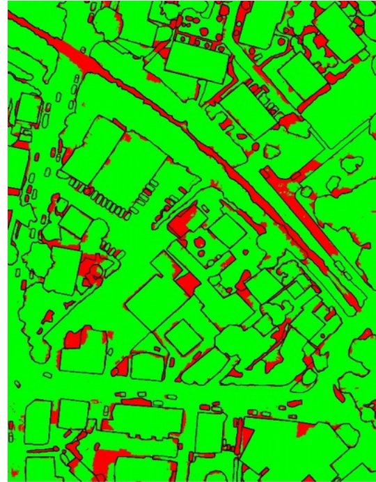
Figure 8: Results from SVL_3: SVL-features, including NDVI, saturation and normalized height, but only boosting classification
