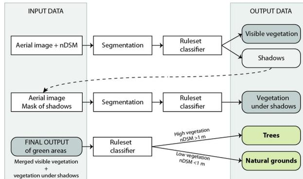
Figure 3. Workflow for urban vegetation extraction with object-based approach.
