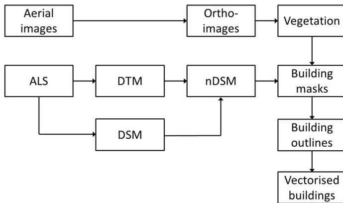
Figure 1. Flowchart of the building extraction.
