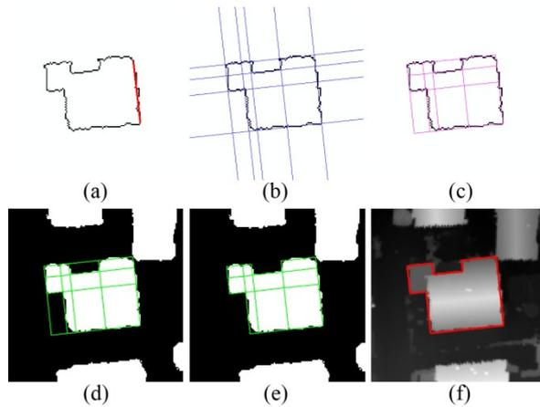
Figure 1. Rectangular building vectorisation procedure.
