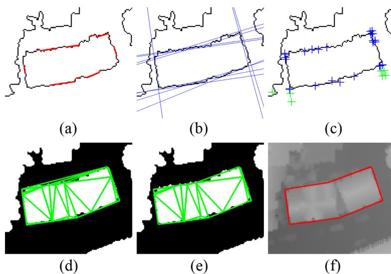
Figure 2. Non-rectangular building vectorisation procedure.
