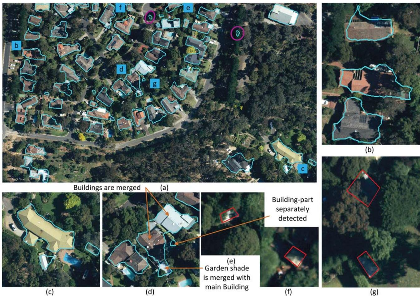
**Figure 9.** Building detection on (a) Area 3 of the VH data set and (b) Area 2 of the AV data set. Building detection examples in: (c–f) Area 2 of the AV data set; and (g,h) Area 3 of the VH data set. Areas marked by letters in (a) and (b) are magnified in (c) to (h).
