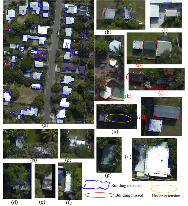
Figure 8. (a) Building detection on AV data set, (b)-(g) Magnified version of the buildings detected under complex scene, (h)-(i) Boundary over-extension, (j)-(m) Undetected buildings, (n)-(p) Boundary under-extension
