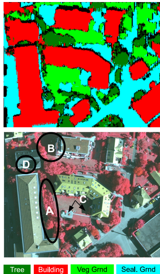
Fig. 6. Area 1: Example for the most prominent type of misclassification: trees and ground vegetation is confused (A, both RTrees and MRF), ground vegetation is classified as ground sealed (B, mainly MRF). Label image from MRF classification. Example for segmentations in (C) and (D), see text. For the colored figure please refer to the online version of this article.
