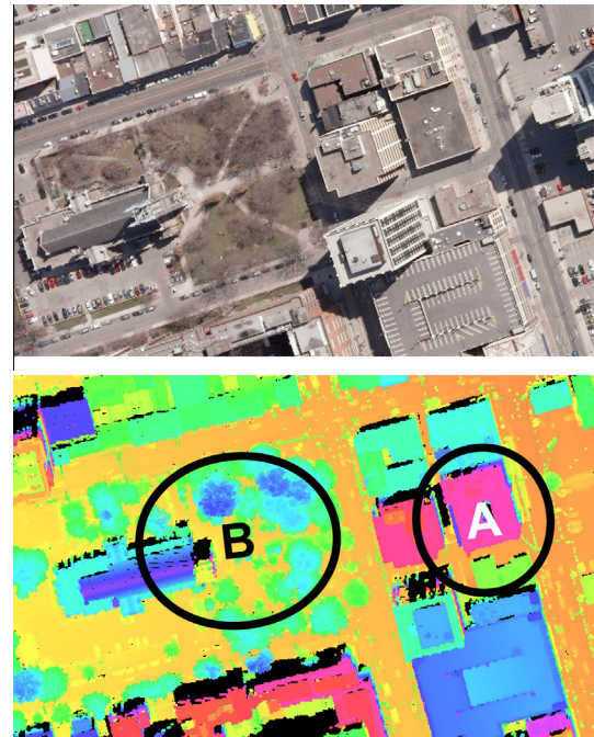
Fig. 11. Examples showing large time difference between ALS and image flight (A), also both flights were done in different vegetation periods (B). For the colored figure please refer to the online version of this article.
