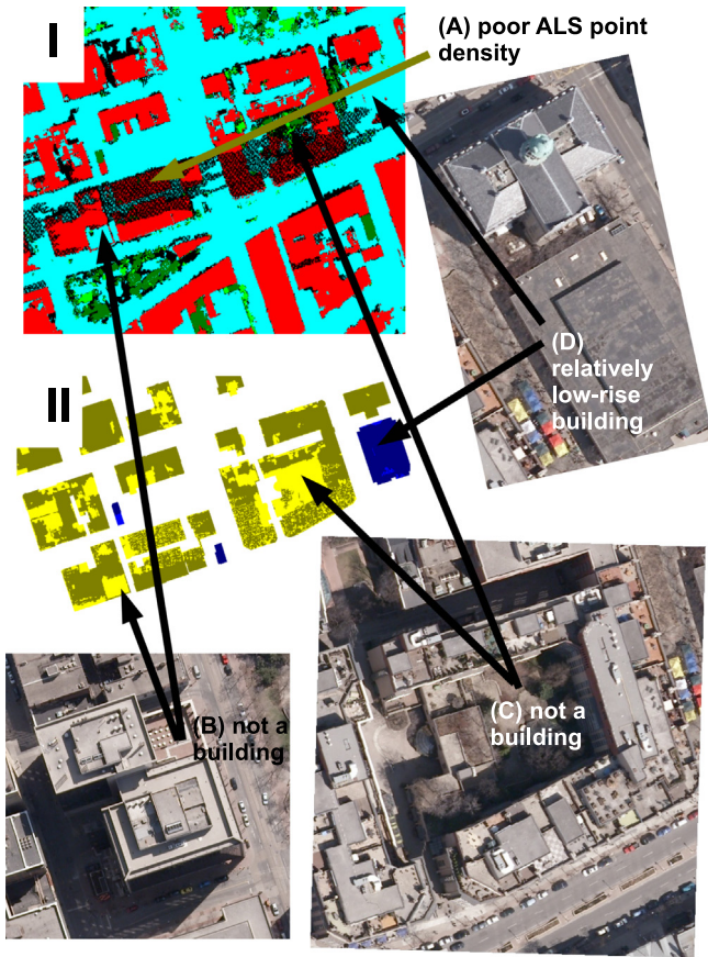
Fig. 13. Area 4: I: labels from RTrees classification (buildings and sealed ground), II: evaluation from ISPRS benchmark, yellow: false negative pixels (but object detected), green: true positive pixels, blue: false negative pixels (and object missed). (A) Shows that the point density is varying in this area, (B and C) show errors in the reference: those spots actually show no buildings, (D) low-rising building which is missed in the RTrees result. For the colored figure please refer to the online version of this article.
