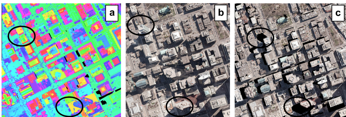
Fig. 1. Example for visibility check, images from the Toronto dataset, see Section 4.2 for a description. (a) Complete ALS point cloud, (b) aerial image (cut out), (c) only points corresponding to visible parts in the image, color grabbed from the image, black parts (also circles): non-visible areas. For the colored figure please refer to the online version of this article.
