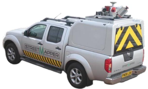
To obtain accurate 3D models for building facades and looking into road conditions, IGI and the British firm 3D Laser Mapping joined forces to build a mobile LiDAR system, *StreetMapper*. *StreetMapper* links laser and camera technology with a high-precision positioning system, *TERRAcontrol*.
