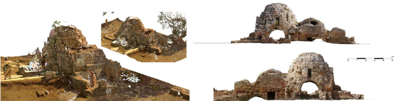
3D point cloud (left), east and west orthophoto (right) of the Mezzagnone building
