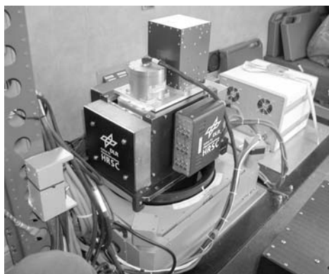
Figure 1: Installation of the HRSC-A with APPLANIX AIMU and IGI IMU-IIId.
