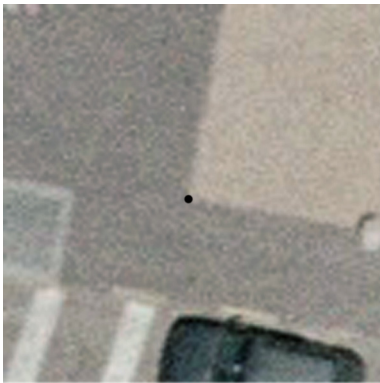
Figure 13: visibility of the PV_NGCP_403 marker on a 1:5000 image.
