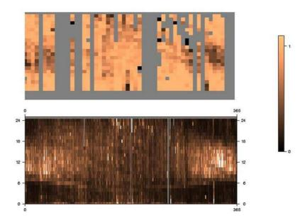
Figure 7: Up: ratio of the number of the  $\Delta \nabla STEC$  values below 2.7 cm. at the station BELL Down: *TEC drift rate* showing the presence of TIDs: In both pictures the x-axis represents days, and the y-axis the time in hours.
