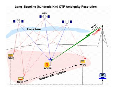
Figure 2: Conceptual picture of the WARTK technique while sending the ionospheric corrections.
