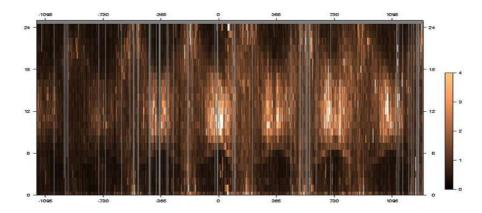
Figure 8: Ratio of the number of the  $\Delta \nabla STEC$  values below 2.7 cm. at the station EBRE since the year 1996. The x-axis represents days, the 0 days corresponds to the 1<sup>st</sup> January 2000, and the y-axis the time in hours.
