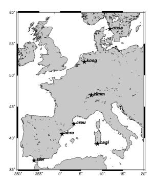
Figure 3: Map of the continental network used in the IONEX comparison. Note that MNTC is the reference station for the double differences.
