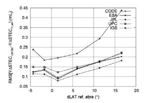
Figure 4: In the right hand side it is depicted the RMS of the  $\nabla\Delta$ STEC as a function of the distance to the reference station EBRE. In the left hand side the same RMS is depicted as a function of the latitude difference to the reference station EBRE.
