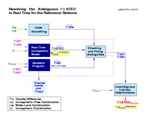
Figure 1: Algorithm scheme for the WARTK technique.
