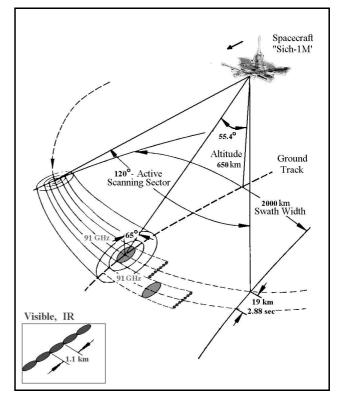
Fig. 2. MTVZA-OK scanning geometry.
