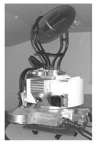
Fig 1. Optical-microwave imager/sounder MTVZA-OK.
