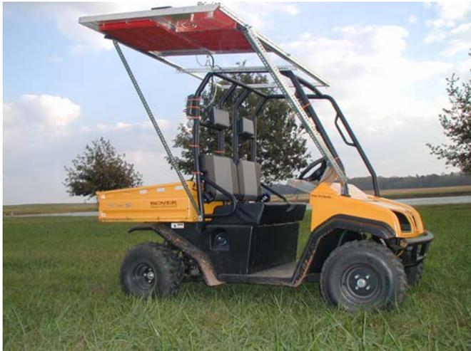
Figure 7. Specialized “Rover” based mobile platform with 3 radiometers, DAS and GPS system on board.
