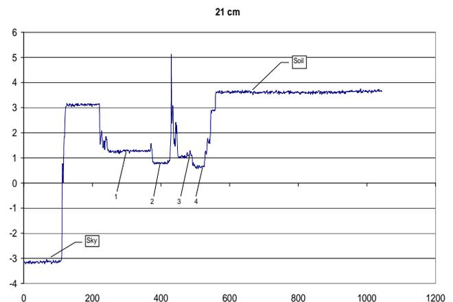
Figure 2. Signals (in volts) at the output of 21 cm radiometer when observing sky, dry land and selected dry soil areas.
