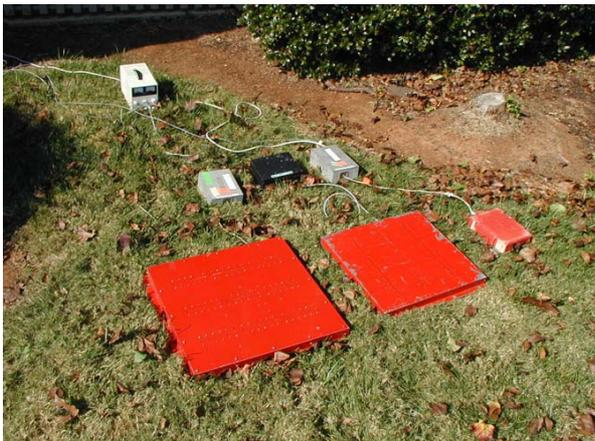
Figure 1. External view of the Geoinformatic/IRE RAS microwave radiometers, operating at the wavelengths of 6 cm, 18 cm and 21 cm.
