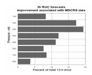
Figure 9. Percentage of 3hr forecast improvement due to aircraft (MDCRS) data.
