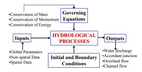
Fig.1 General theory and workflow to construct DHM
