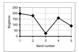
Figure 1. Typical spectral dependence of brightness of a snow cover from NOAA data.
