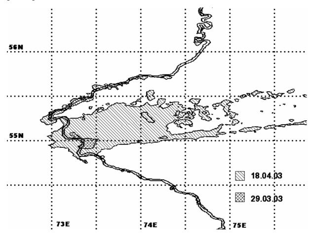
Figure 2. Borders of territory free from a snow cover in the beginning and at the end of the period of thawing - March 29 and April 18, 2003 accordingly. The small internal contour (index 2) corresponds to the beginning of the period of thawing. The large external contour (index 1) corresponds to the ending of the period. For simplification of orientation in figure the contours of the river Irtish are given.
