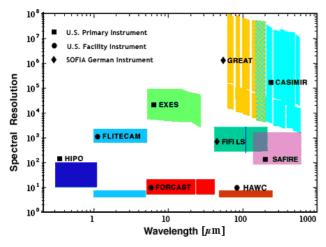
Figure 3. Spectral resolution and wavelength of SOFIA instruments.
