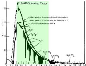
Figure 2 Solar Spectrum (intensity vs. wavelength) and EnMAP operation range.
