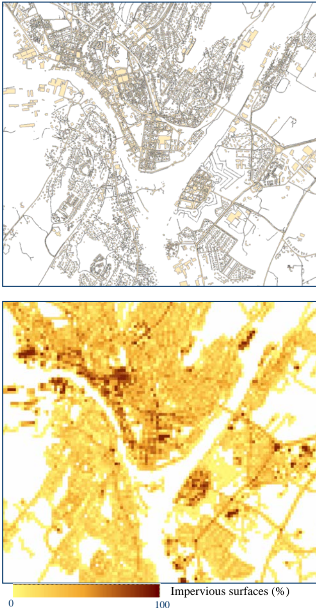
Figure 2. Reference data generated by rasterizing high resolution polygon map data of buildings and roads to 30 m pixels. The image extract shows the center of the city Fredrikstad.
