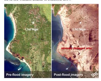
Figure 2. Change detection for Lho'Nga after Tsunami hit the area on December 26, 2004; Ikonos imagery of January 29, 2003 (left) and December 29, 2004 (right); blue line indicate former shoreline, red lines represent recent shoreline and damaged area (Image Source: CRISP Singapore)
