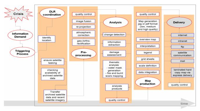
Figure 1. DLR Rapid Mapping Service - processing chain
