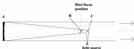
Figure 1. The coaxial Newton telescope design of Axelsson et al. 1990
