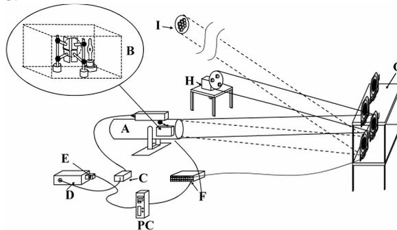
Figure 2. Experimental setup of an entire Multibeam system (Pundt and Mettendorf, 2005)
