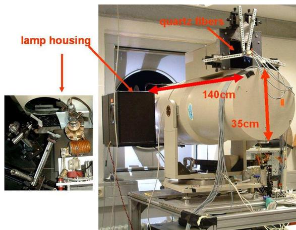
Figure 3. Multibeam Long path DOAS instrument (Hydra). Extended view: inside of the lamp housing from above
