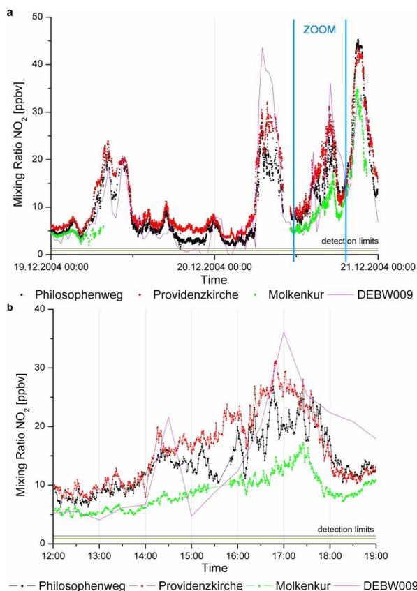
Figure 6a)  $\text{NO}_2$  average mixing ratio measured during two days along three different light paths together with results from in situ measurement “DEBW009”; b) 7 hours zoom from plot a)
