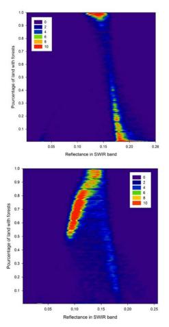
Figure 6 a) Percentage of forest contained in a 990m pixel based on LANDSAT ETM+ 90x90m area in function of the SWIR band reflectance at 990m for a) area with no water, and b) areas with water. Other bands gave similar results.
