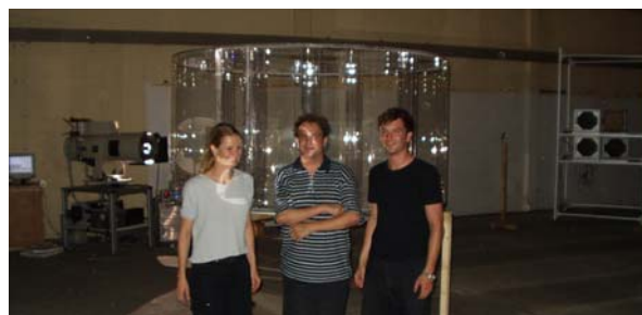
Figure 7. Picture of the Tom-DOAS validation experiment. One Multibeam-system (left), one polycarbonete cell (middle), and one mirror tower (right side) can be seen. Four light beams from another telescope are directed onto the experimentalists.
