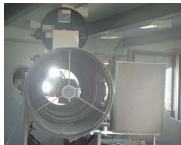
Figure 6. Picture of the Multibeam telescope from the front. Two virtual lamps appear on the telescope main mirror.
