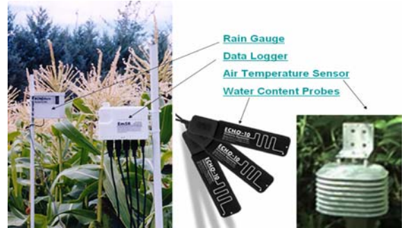
Figure 1. Instruments of a soil moisture station.
