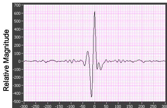
Figure 4. The central portion of an interferogram of a warm blackbody source with both the high and low gain channels combined.
