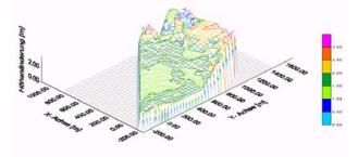
Figure 3: Swiss Camp, volume decrease from digital elevation models, difference 2004 minus 2002 (X-Axis = NORTH, Y-Axis = EAST)
