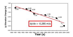
Figure 2: Swiss-Camp, elevation change of ice horizon for all 4 stakes.
