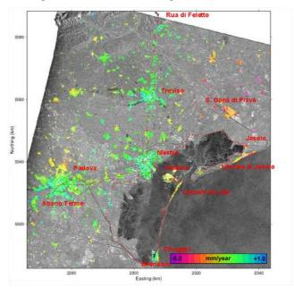
Figure 4. INSAR land subsidence map (in mm/year) of the Lagoon of Venice for the time period 1993-2000 with ground based levelling network superimposed
