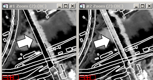
Figure 3. Orthoprojection with a DEM (left) and with a Dense DEM (right)
