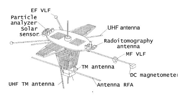
Fig.1. COMPASS microsatellite
