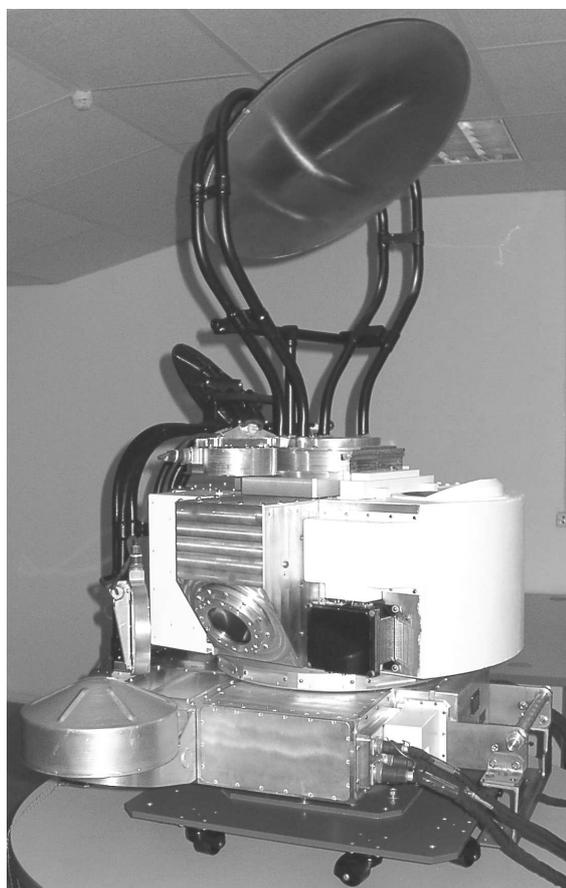
Fig 1. Optical-microwave imager/sounder MTVZA-OK.
