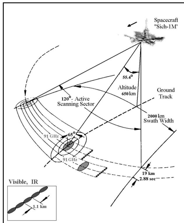
Fig. 2. MTVZA-OK scanning geometry.
