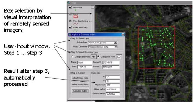
Figure 3. Case of connectivity analysis with satellite imagery in a rectangle region.
