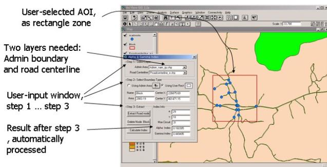
Figure 2. User interface of connectivity analysis on the GIS layers, and the processing steps.
