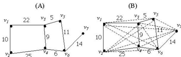
Figure 6. (A) Example of Road network with distance, (B) Fully connected road graph network.
