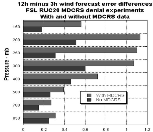
**Figure 8. Differences between 12hr and 3 hr forecasts with and without aircraft (labeled MDCRS) data. Difference in RMSV Error shown in  $m s^{-1}$ , where  $1 m s^{-1}$  equals approximately 2 knots.**
