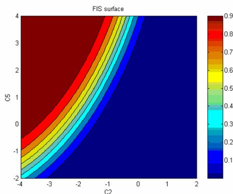
Figure 4. FIS surface of the ANFIS model. Colours from blue to brown identify low to high membership values.
