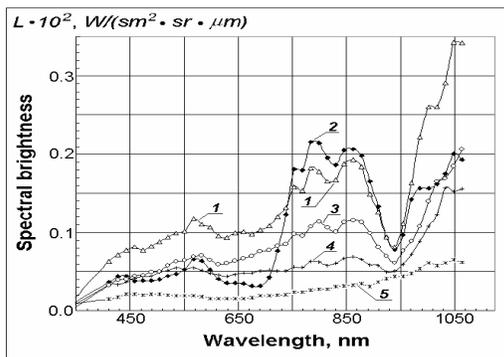
Figure 2. Brightness spectra received by spectroradiometer for various types of surfaces: 1–field vegetation; 2–healthy fir-tree forest; 3, 4–fir-tree forest with the different degrees of trees burning-out; 5–completely burned-out forest.
