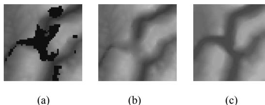
Fig 3. The DEM data in the rectangle of fig2. (a) Raw SRTM data (black represent voids); (b) The patched SRTM data; (c) TopoDEM
