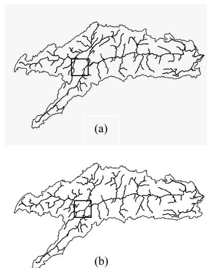
Fig 2. The drainage network and catchment boundaries derived from DEM datasets. (a) SRTM DEM; (b) TopoDEM
