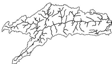
Fig 4. The drainage network and catchment boundary derived from SRTM DEM datasets with new patching method
