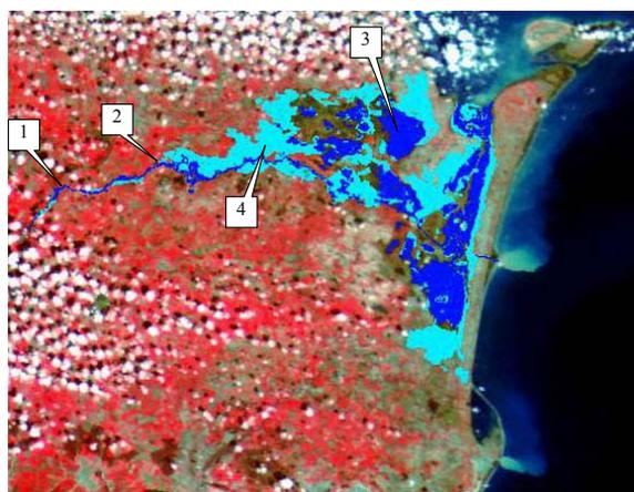
Figure. 5. Inundation of the Terek delta during catastrophic flush on the basis of RSD.
