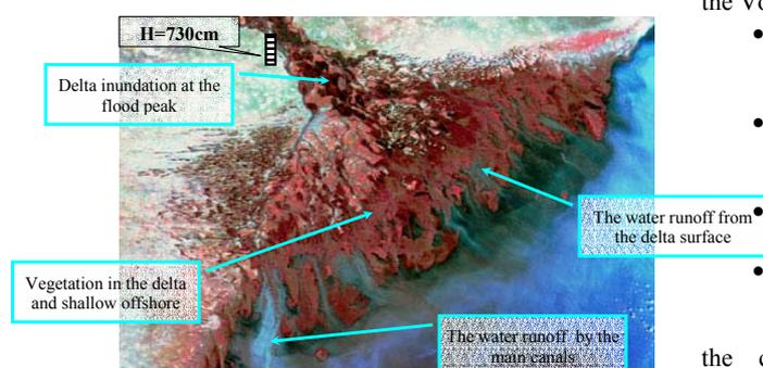
Figure 4. Inundation during the flood peak in 2002 according to RSD
