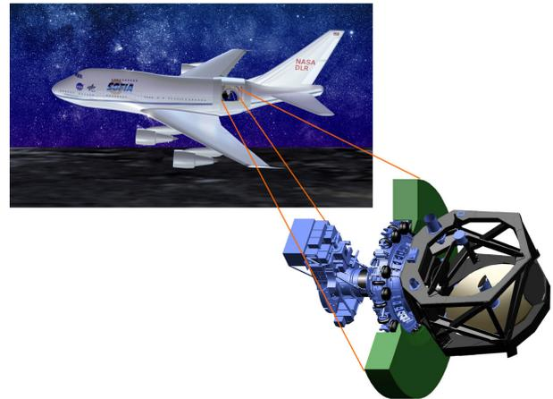
Figure 1. SOFIA and its telescope.
