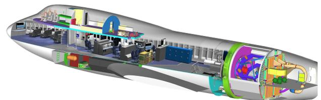
Figure 2. Cut-away view into the SOFIA aircraft
