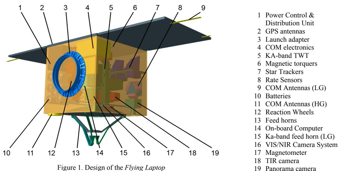
Figure 1. Design of the *Flying Laptop*
