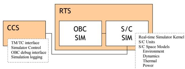
Figure 6. Block diagram of the Software Verification Facility
