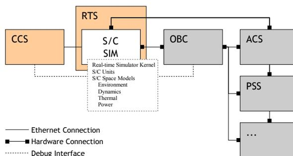
Figure 7. Block diagram of the FlatSat test bench which integrates flight hardware (grey shaded) in the simulation loop
