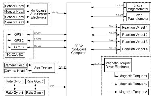
Figure 3: ACS block diagram
