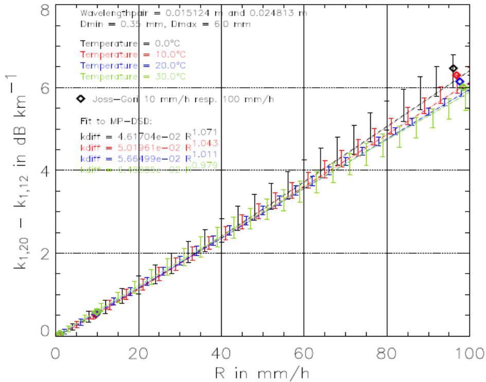
Figure: 4 [4]: Attenuation  $\Delta k_i$  (20GHz - 12GHz) [dB/km] versus rain rate [mm/h] calculated for different drop size distributions (error bar) and temperatures (color). The rain rate refers to the speed of drop fall at sea level.
