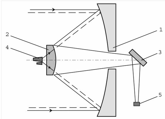
Figure 2. The Ka-band and the thermal infrared camera, use a cassegrain system which is designed as a dual band system: (1 – primary mirror, 2 – secondary mirror, 3 – beamsplitter, 4 – feedhorns, 5 – TIR camera)
